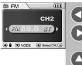
1.Press the left or right button to adjust frequency until you find the desired station.(If you find a channel that appear clearly, it will show "ST" on the screen, or it shows "MO")
